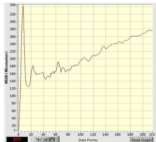
Figure 5. Wear Rate of Pure Aluminium 97% + 3% Diamond
