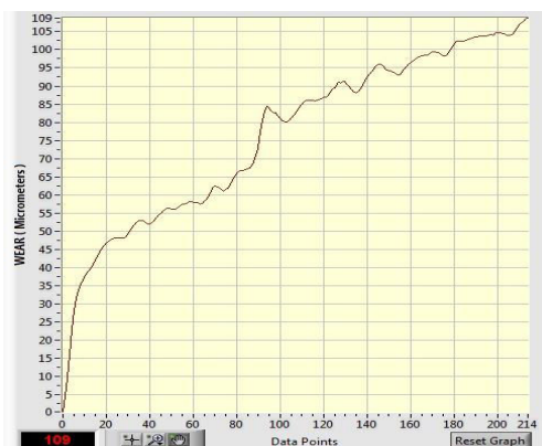
Figure 3.Wear Rate of Pure Aluminum
